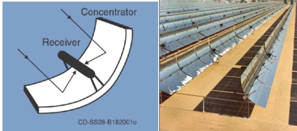
Fig 1 : Parabolic Trough System Schematic Diagram & Parabolic trough system
